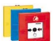
The **MCP 535 manual call point** is used to manually trigger a fire alarm (type B in compliance with EN 54-11). The detector is fitted with an integrated short circuit isolator as standard and can be individually disabled. Any language can be quickly and simply selected by using interchangeable descriptor strips, with the detector available in various versions (various IP protection categories and colours).
