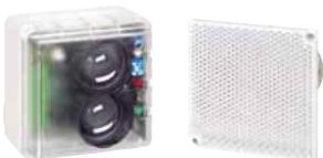
The **ECO linear smoke detector** consists of a combined transmitter and receiver unit and a reflector which are fitted opposite one another. The infrared beam that is emitted by the transmitted is reflected and evaluated. The detector is particularly suited to being used in historical buildings, museums, hotels etc. on account of the low amount of wiring it requires.
