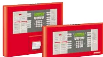
The **MMI-CIP and MMI-CPP external operating panels** can be connected to the Integral, Integral C and Integral C1 fire alarm control panels. Up to 8 external operating panels can be connected to a sub control unit via its own data bus, with a maximum distance of up to 1,200 m to the sub control unit. User interfaces and display texts are available in 20 languages. Dimensions (H x W x D): 230 x 445 x 35 mm or 360 x 445 x 45 mm (with printer).
