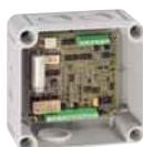
The **BA-OI3 input/output module** contains a relay output with a programmable fail-safe position, two inputs for querying potential-free contacts and an optocoupler input for monitoring external voltages. The module contains a short circuit isolator and is primarily used for connecting special detectors to the loop circuit technology.
