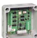
The **BA-IM4 input module** contains 4 inputs for the monitored and non-monitored querying of potential-free contacts, as well as an integrated short circuit isolator. The inputs are suited to detecting switching states of more than 330 ms, with the operating mode being configurable and which can be set separately for every input.
