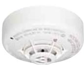
The **DCD-1E-IS temperature detector** is a conventional class 1 maximum and change in temperature detector, with an additional fixed alarm threshold at 60°C and is designed especially for use in hazardous areas. The detector is connected to the Integral loop circuit using a BA-AIM branch module and a Zener barrier and contains 2 LEDs positioned opposite one another for indicating an alarm. The detector is approved for use in class 1 and 2 hazardous areas.
