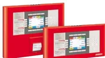
The **High-End Operating Panel** with a VGA colour display and function keys allows the easy operation of a fire alarm system and offers a structured overview of complex SecoNET fire alarm networks. The user interface and display texts are available in 20 languages. Dimensions (H x W x D): 230 x 445 x 35 mm or 360 x 445 x 45 mm (with printer).
