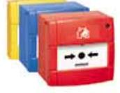
The **MCP 545 manual call point** is used to manually trigger a fire alarm (type A in compliance with EN 54-11). The detector is fitted with an integrated short circuit isolator as standard and can be individually disabled. The alarm is triggered by smashing the glass panel, with the detector being available in different versions (IP protection class and colour).
