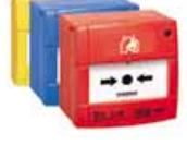
The **WRIS manual call point** is used to manually trigger a fire alarm in hazardous areas (type A in compliance with EN 54-11) and is ATEX approved. The alarm is triggered by smashing the glass panel, with the detector being available in different versions (IP protection class and colour).
