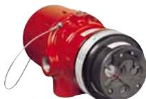
**Flame detector for hazardous areas** in a case tested in a hazardous area, available as UV, infrared or combined UV/IR detectors. The detectors are suitable for outdoor use, and are particularly suitable for use where flames are concealed by smoke thanks to the unit's own particular optical self-monitoring process. All versions are not sensitive to sunlight, with larger flames being detectable from greater distances. All detectors are approved in accordance with ATEX 100a and VdS.
