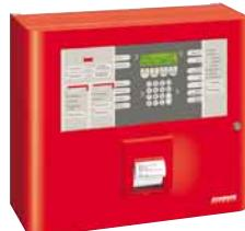
The **BMZ Integral C1** is a non-modular non-networkable small-scale control panel for connecting a single loop circuit with up to 128 devices. The BMZ Integral C1 is available either with or without a log printer. Furthermore, external operating panels and fire brigade control panels can also be attached. The unit is programmed using a laptop and the user interface and display texts are available in 20 different languages.
