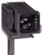
The **ARDEA linear smoke detector** consists of transmitter and receiver units and is suitable for monitoring areas of up to 3000 m<sup>2</sup>. Detection occurs based on an absorption measurement whilst taking dynamic parameters (smoke modulation) into account, with the detector also set to the flame frequency of an open fire. The ARDEA is also available in special versions for use in hazardous areas and with IP 65 protection class.
