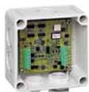
The **BA-AIM branch module** is used to connect conventional D/C detectors to the loop technology or as a branch unit for monitoring hazardous areas. It contains a monitored input, a parallel indicator output and a short circuit isolator.
