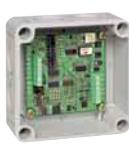
The **BA-IOM input/output module** is used, for amongst other things, to control monitored devices, which are supplied with power by an external power supply (e.g. sirens etc.). It contains a short circuit-proof monitored output and a galvanically isolated input, as well as an integrated short circuit isolator, with the power supply also being internally monitored on the loop circuit for undervoltage.
