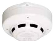
The **SLR-E-IS optical smoke detector** is designed specially for use in hazardous areas and is connected to the Integral loop circuit using a BA-AIM branch module and a Zener barrier. The detector contains 2 LEDs positioned opposite one another for indicating an alarm and is approved for use in class 1 and 2 hazardous areas.
